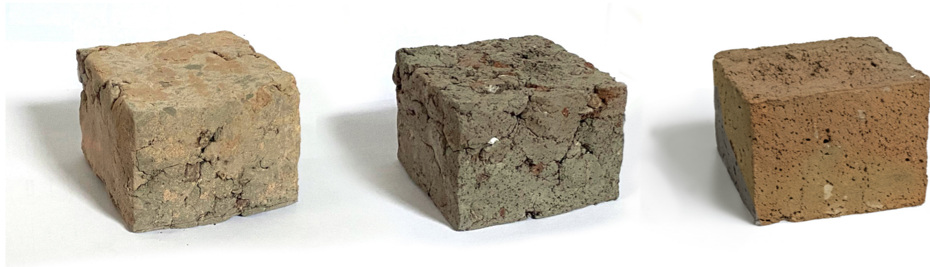
External Structural Fired Earth Brick
